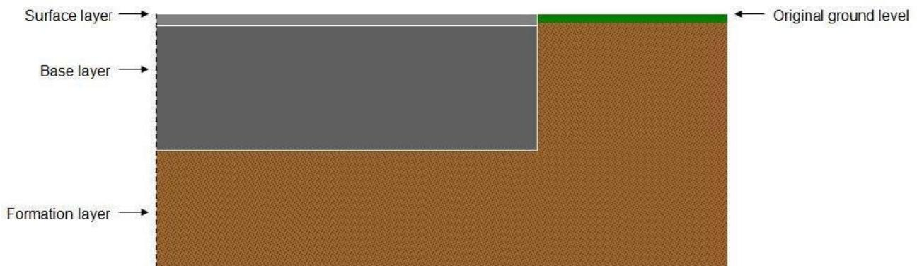
If the ground is soft or wet, the path is typically raised slightly above adjacent ground level to allow all water to run-off the path surface and into the adjacent ground or drainage feature.
