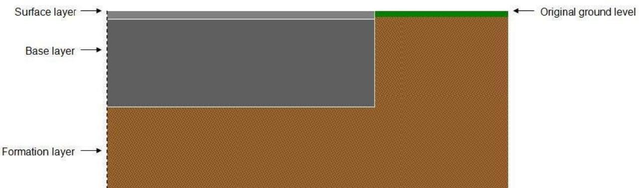
If the ground is soft or wet, the path is usually built-up above ground level to prevent water running back on to the surface. In the diagram below, you will see that the surface layer now sits above the original ground level. We call this a **half-tray**.
