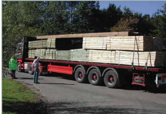
Delivering long beams to site can require access for large vehicles
